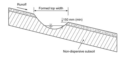
(a) Parabolic catch drain with down-slope bank
